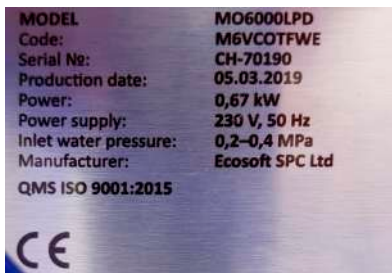
Figure 31. RO machine nameplate
