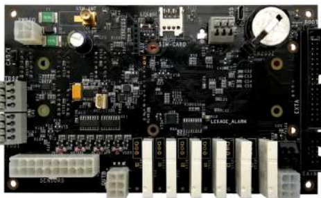
Figure 30. Battery connector on OC6000 PCB
