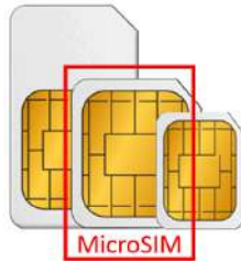
Figure 22. Required type of SIM-card — MicroSIM
