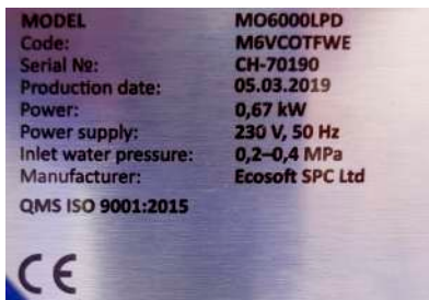
Figure 31. RO machine nameplate
