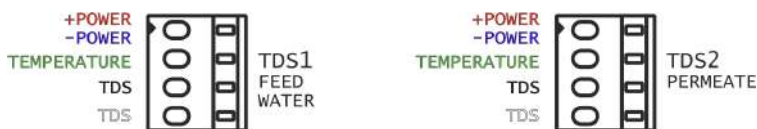
Figure 4. Inputs of OC6000 — TDS1 and TDS2 connectors for combined electrical conductivity & temperature sensors
