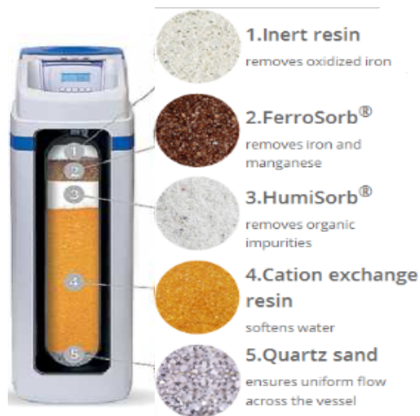
Fig. 2.13. Ecomix multi-component filter material
