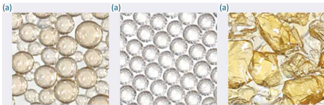
Fig. 2.3. Ion-exchange resins of polymerization (a, b) and polycondensation (c) types; polydisperse (a, c) and monodisperse (b) granulometric composition
